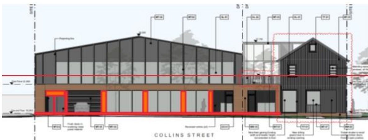
Figure 28: Suggested details (highlighted red and inserted by Council officer) showing increased masonry columns to the Collins Street facade.
